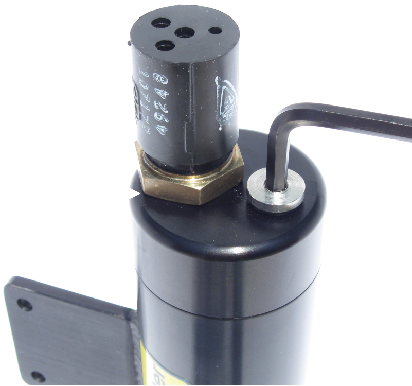
Figure 1 – Removing the Oil Compensation Plug
